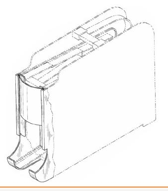
The Samways reference discloses a dispenser with "a serpentine delivery path . . . along which cylindrical objects to be dispensed can move under the action of gravity."
